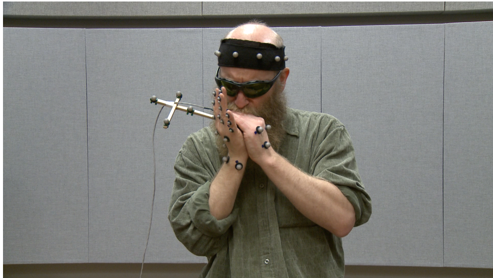
Fig. 4.1 – John is playing the modified harmonica, with markers attached to his hands and wearing a marker head band.
