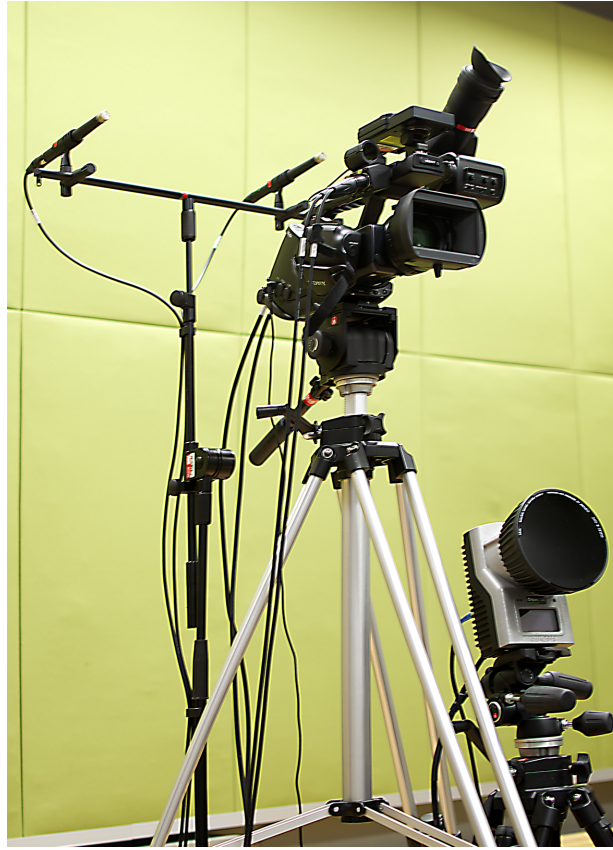
Fig. A.3 – Left to right: DPA 4006-TL Stereo Microphone set, Sony PWM EX-3 professional high definition video camera, Qualisys Oqus motion capture camera with high-speed infrared video capture.
